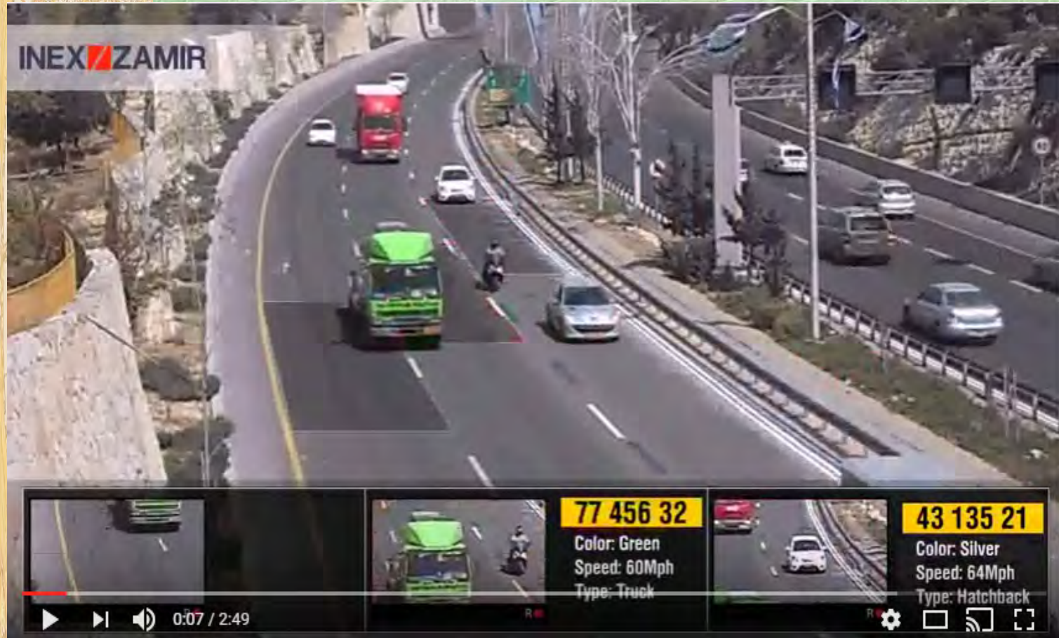
Figure 5-6: Application of ALPR for Traffic Management
