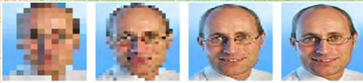
Figure 1-20: Effects of Pixels-on-Target on Image Quality
