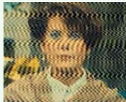
This image is the result of an interference issue
