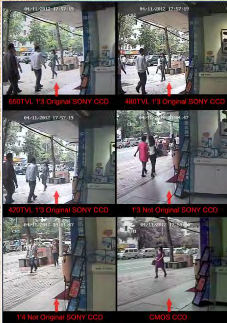
Figure 1-15: CCD and CMOS Camera Lens Comparison
